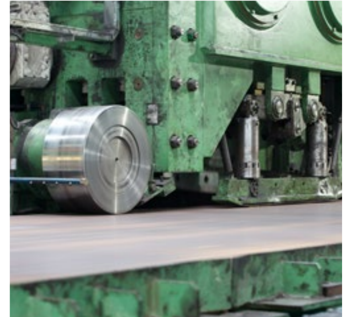
Double side trim shear at Dongkuk Steel, Dangjin, South Korea
