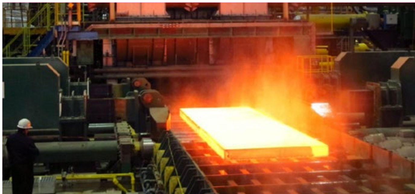
Plate-Steckel mill at AHMSA, Monclova, Mexico
