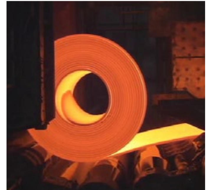
Coil box at Baosteel Stainless Steel Co., Ltd. Shanghai, China
